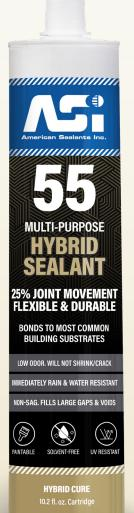
ASI 55 is used for Industrial & Commercial Construction. This one-part, moisture cure, Hybrid Sealant and Adhesive cures to form a permanent, durable, rubber for use in various adhesive and sealant applications. It works well on Galvanized Steel, Stainless Steel, and Aluminum. It has a service temperature of -50° F to 220° F, skin formation time of 30 minutes (at 70° F, 50% RH), and 300% elongation at break.
