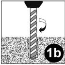
**Traditional Drilling Method for dry and damp concrete** - Using a rotary hammer drill, and a bit which conforms to ANSI B212.15 and is the appropriate size for the anchor diameter to be installed, drill the hole to the specified embedment depth. **CAUTION:** Always wear appropriate personal protection equipment (PPE) for eyes, ears & skin and avoid inhalation of dust during the drilling and cleaning process.
