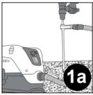
**Recommended Dust Extractor System for drilling into dry concrete** - Attach appropriate size drill bit to the Dust Extractor Vacuum System (see Table 2). The drill bit should conform to ANSI B212.15 and be the appropriate size for the anchor diameter to be installed. Drill the hole to the specified embedment depth. Skip to Step 5 if using Dust Extractor System.
