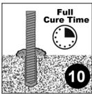
Do not disturb, torque or apply any load to the installed anchor until the specified full cure time has passed. The amount of time needed to reach full cure is base material temperature and moisture dependent - refer to Table 5 for appropriate full cure time.
