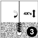
Select the correct wire brush size for the drilled hole diameter (see Table 3), making sure that the brush is long enough to reach the bottom of the drilled hole. Reaching the bottom of the hole, brush in an up/down and twisting motion for 4 cycles (4X). **CAUTION:** The brush should contact the walls of the hole. If it does not, the brush is either too worn or small and should be replaced with a new brush of the correct diameter.
