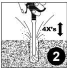
**NOTE:** Remove any standing water from hole prior to beginning the cleaning process. If removal of standing water is not possible, please contact ATC for application specific installation instructions. Using oil free compressed air with a minimum pressure of 80 psi (5.5 bar), insert the air wand to the bottom of the drilled hole and blow out the debris with an up/down motion for a minimum of 4 seconds each cycle (4X).
