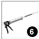
After the cartridge has been prepared, screw on the proper ATC mixing nozzle to the cartridge (see Table 1). Do not modify mixing nozzle. Confirm that internal mixing element is in place prior to dispensing the adhesive. Take note of the air and base material temperatures and review the working/full cure time chart (see Table 5) prior to starting the injection process.
