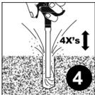
Blow the hole out once more to remove brush debris using oil free compressed air with a minimum pressure of 80 psi (5.5 bar). Insert the air wand to the bottom of the drilled hole and blow out the debris with an up/down motion for a minimum of 4 seconds/cycles (4X). Visually inspect the hole to confirm it is clean. **NOTE:** If installation will be delayed for any reason, cover cleaned holes to prevent contamination.
